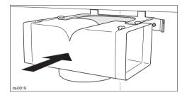
■ Slide the diverter on to the brackets of plate B.
